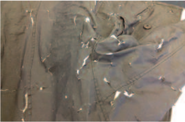
The polyurethane coating became so brittle it cracked.
