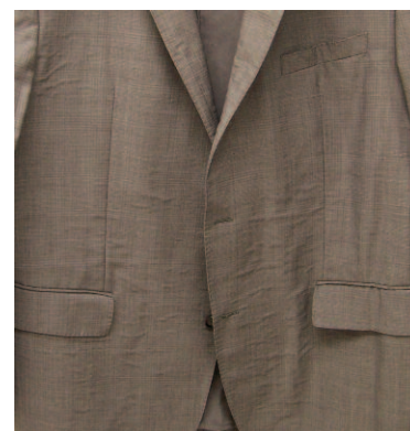
The interfacing bonded to the fronts of this suit jacket separated in cleaning and these areas are now blistered.
