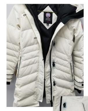
During proper dry cleaning, as labeled, the black trim dve bleeds into the white body section, causing objectionable staining.
